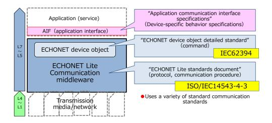
The "ECHONET Lite communication middleware" and "device object detailed specifications", which are the main parts of the ECHONET Lite Specifications, have been certified as international standard specifications by IEC and ISO/IEC.
