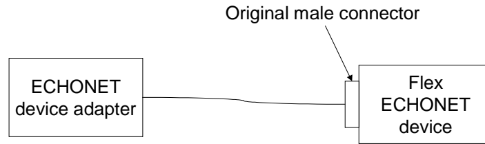
Fig. 3.7 Device/Adapter Connection Example for Type 4 (Open Collector)
