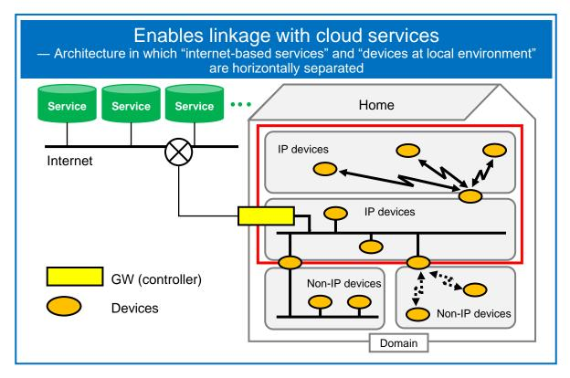
Because the system above can be built, specifications study and development in services and devices can be done respectively and parallelly. This enables us to expect services to be provided not only by device manufacturers but also by various service providers.
