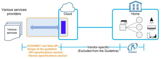
The ECHONET Lite Web API Guidelines are composed of two types of documents: (1) API specifications section that summarizes the definition policies of the Web API models and the mapping policies from ECHONET Lite specifications; and (2) Device specifications section that summarizes the Device Description for each device.
